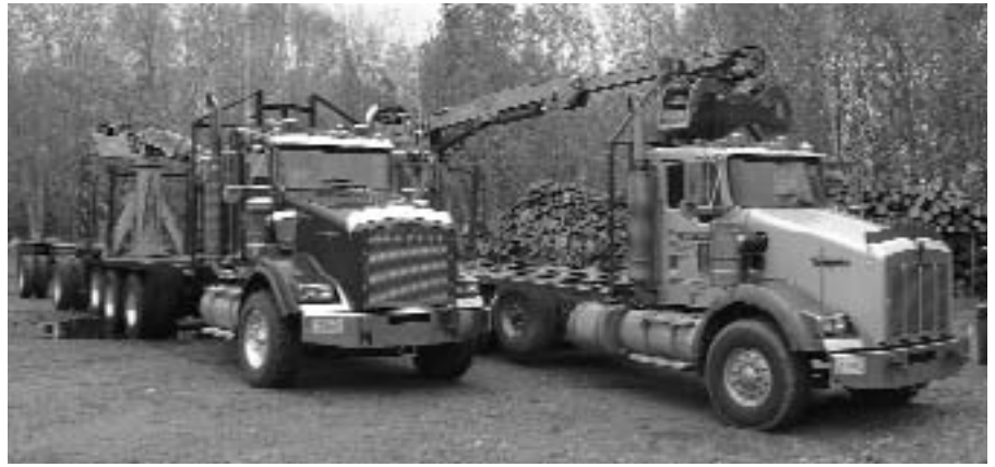
Two of the trucks DeMenge uses to haul wood. They’re Kenworth trucks with pup trailers and Serco loaders. DeMenge also owns a Hydroax 411 feller buncher, two John Deere skidders (a 548G and a 440), and a 1989 W900 Kenworth tractor so his sons can cut the stumpage he buys.
