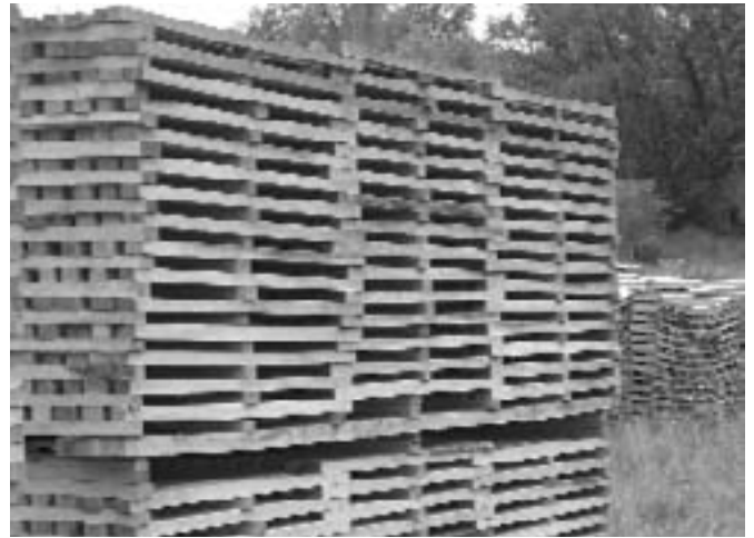
Staves for wine barrels are stacked behind the mill and aged for 24 to 26 months. Staves for whiskey barrels are shipped immediately.
