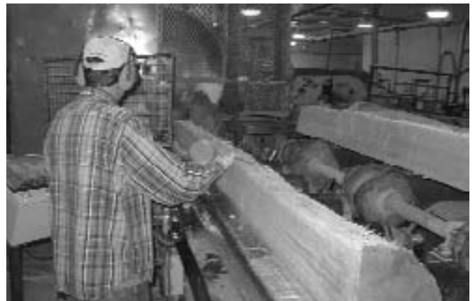
White oak logs are quartered in the mill and then cut to 36-inch lengths. Eventually, the wood is cut into staves measuring 36 by 1-1/2" with random widths.
