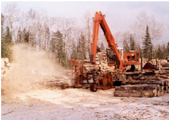
Besides sawdust the slasher operator, Jason Wardas, makes 100-inch wood out of tree-length.
