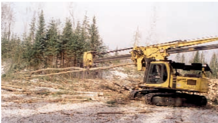
The delimitter operated by Tim makes quick work of delimiting and topping another hardwood tree.
