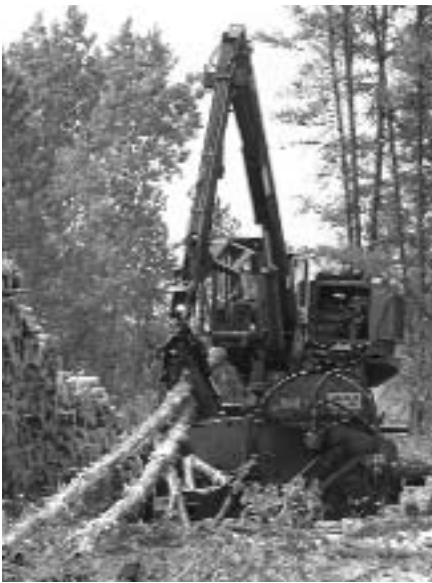
The Hood S182 slasher is operated by Scott Morrison, who cuts and stacks the wood before it's hauled to the mill.
