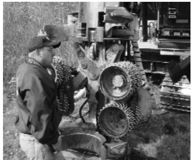
Sean Petty explains the processor head. The roller that they use to measure sticks is the vertical silver piece in the middle of the processor head, just about level with Sean's head.
